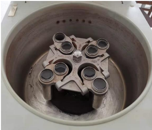
Fig. 3 Desalination treatment of marine dredged clay by centrifugation
