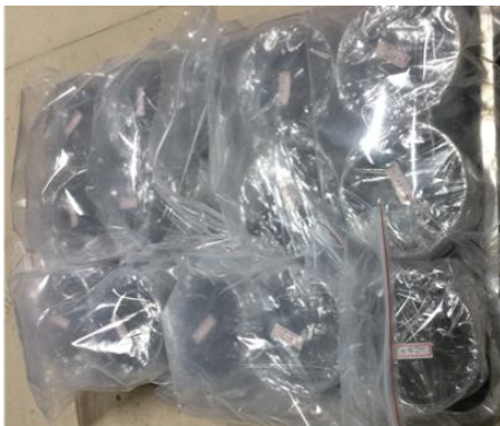
(a) Plastic cups containing treated dredged clay
