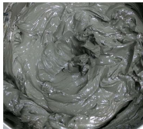
Fig. 2 Marine dredged clay after mixing
