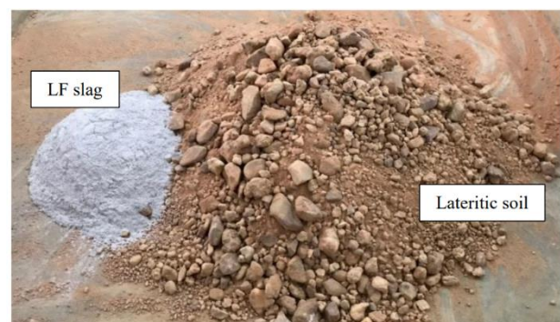
Fig. 3 Ordinary lateritic soil with 10% LF slag
