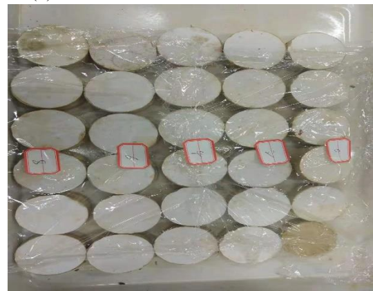
(f) Soil samples for dry-wet cycling tests
