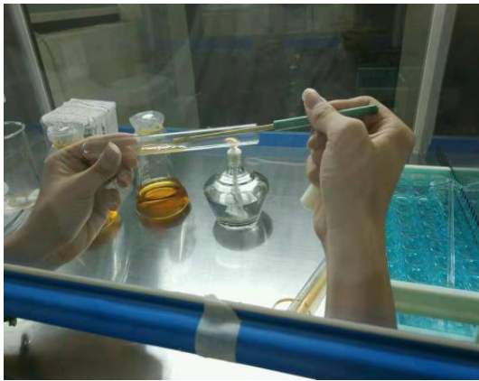
(a) Inoculate with Sporosarcina pasteurii
