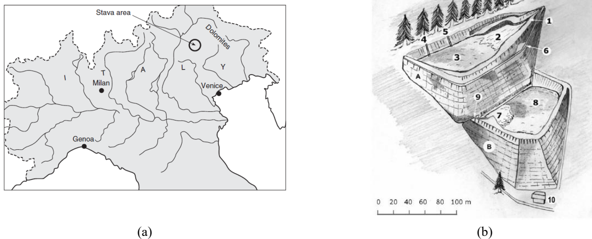
Fig. 4 Stava basins. (a) Geographical localization and (b) sketch: A upper basin, B lower basin, (1) on-dam cyclone for the extraction of the coarser sand components from the tailing wastes, (2) upper beach, (3) upper pond, (4) drainage service, (5) emergency drainage, (6) service road, (7) lower beach, (8) lower pond, (9) drainage from the upper dam, (10) caretaker's house (modified from Luino and De Graff 2012)
