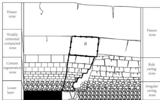
Fig. 4 Distribution of each zone in the regenerated roof
