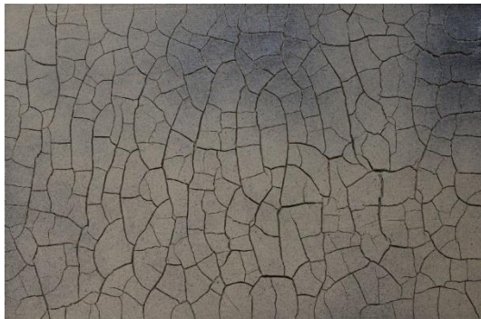
Fig. 6 Typical crack patterns at the end of desiccation (thickness = 4 mm, t = 30 h)
