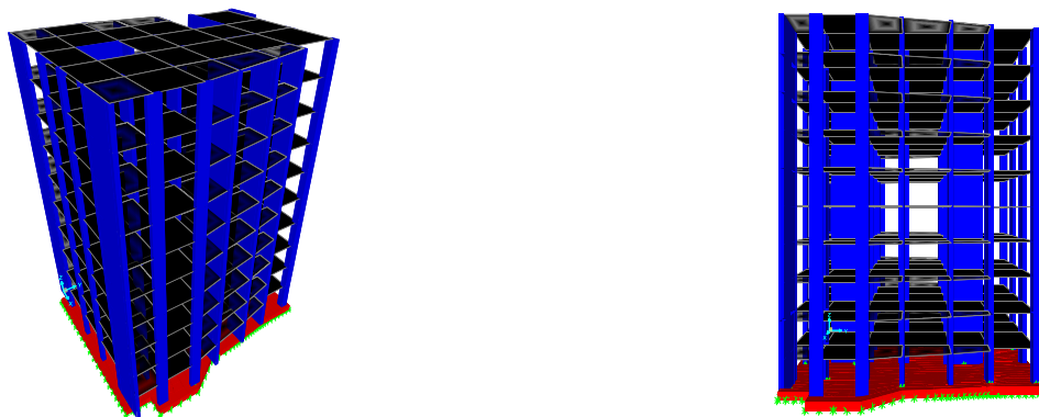
Fig. 8 FE model of R/C building structure
