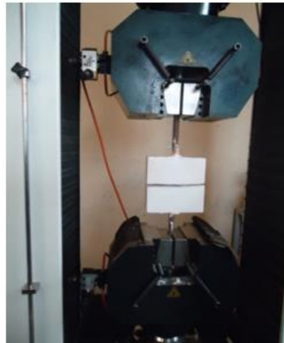
Fig. 3 The model with pre-existing notch in tensile device
