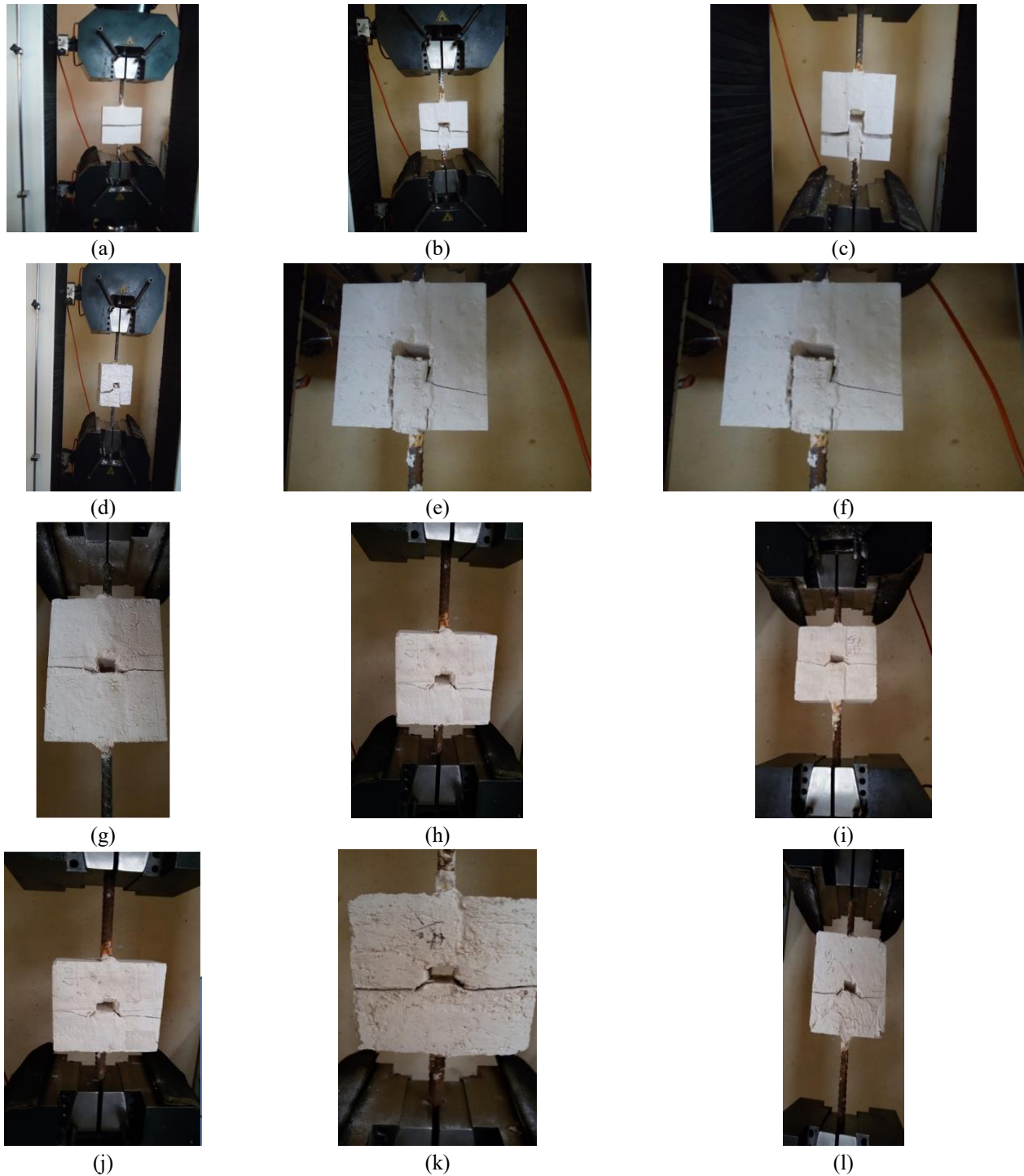
Fig. 4 (a) failure pattern of intact model, (b) failure pattern of model consisting two vertical non persistent notch, (c) failure pattern of model consisting two vertical non persistent notch, (d) failure pattern of model consisting one oriented edge notch with angle of 40 and one persistent notch, (e) failure pattern of model consisting one vertical non persistent notch and one persistent notch; (f) failure pattern of model consisting one vertical non persistent notch and one persistent notch, (g) failure pattern of model consisting two edge notch; h) failure pattern of model consisting two oriented notch; (i) failure pattern of model consisting two oriented notch, (j) failure pattern of model consisting two oriented notch, (k) failure pattern of model consisting two oriented notch, (l) failure pattern of model consisting two oriented notch, (m) failure pattern of model consisting two oriented notch, (n) failure pattern of model consisting two horizontal non-persistent joint; (o) failure pattern of model consisting two horizontal non-persistent joint, (p) failure pattern of model consisting two horizontal non-persistent joint, (q) failure pattern of model consisting two oriented joints and two horizontal notch, (r) failure pattern of model consisting two horizontal edge notch, (s) failure pattern of model consisting two horizontal edge notch, (t) failure pattern of model consisting three oriented joint, (u) failure pattern of model consisting three oriented joint and (v) failure pattern of model consisting three oriented joint
