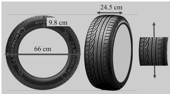
Fig. 3 Scrap tire size and direction of the tensile test
