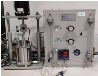
Fig. 2 Pressure plate apparatus used in tests
