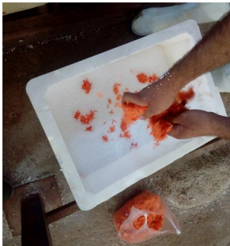
Fig. 2 Adding PP fibers to the geofoam beads fiber used in this study
