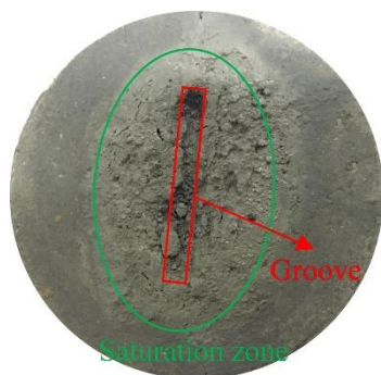
Fig. 16 Schematic of the clay sample after testing
