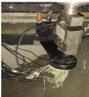
Fig. 5 Single pile testing model at 45 degree slope
