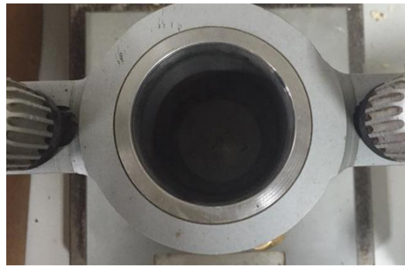
Fig. 4 Specially designed compaction mold
