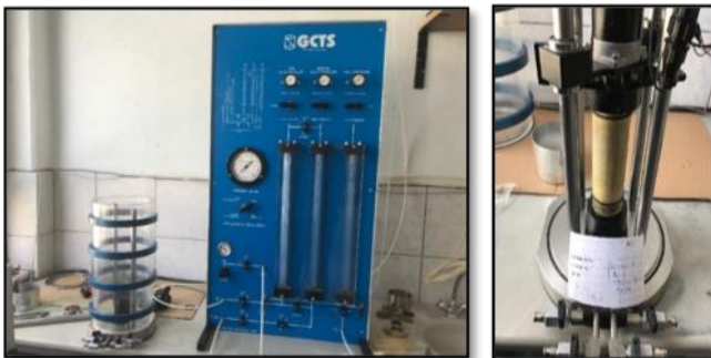
Fig. 6 Demonstration of the Resonant column test system and a soil sample
