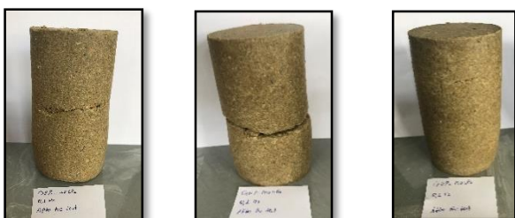
Fig. 7 Deformed samples after TRX experiments
