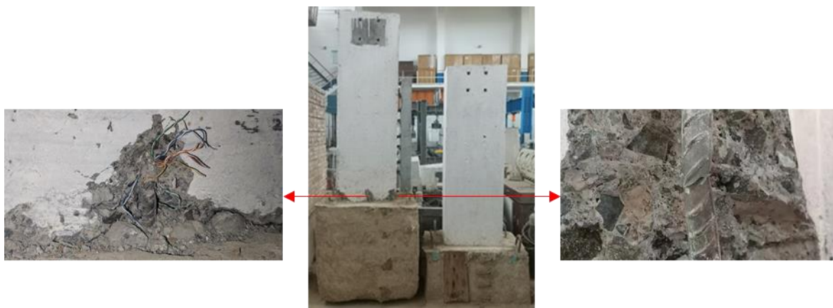
Fig. 16 Comparison of the failure phenomena for the two model piers after testing
