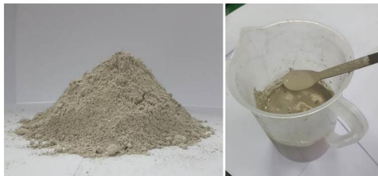
Fig. 3 Micro cement for grouting injection: Powder (left), Fluid mixture (right)
