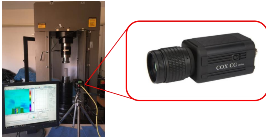
Fig. 1 MTS 815 test system with COX thermal camera
