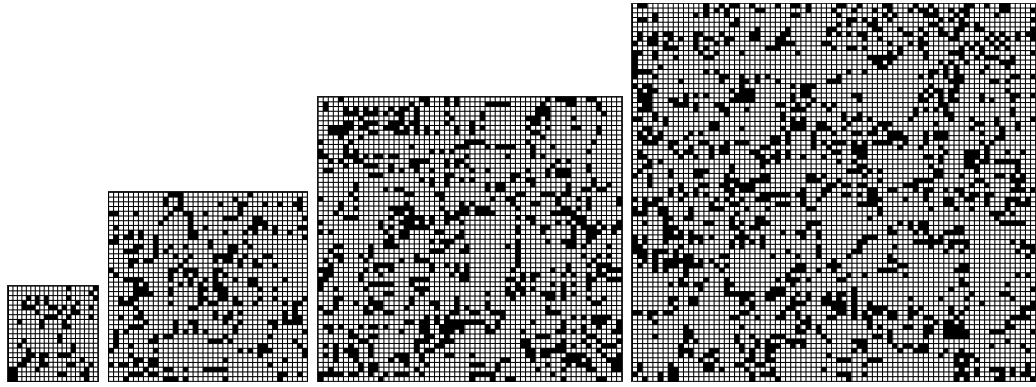
Fig. 5 Numerical models of different sizes for random field with L = 10 and n_p = 20\%
