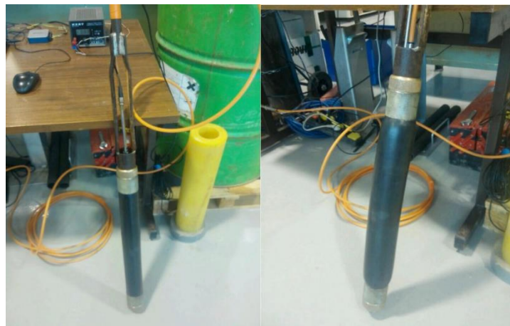
Fig. 15 Pressuremeter probe during the calibration phase
