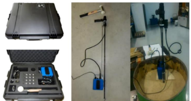
Fig. 18 Overview of the PANDA 3® Labo Penetrometer
