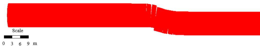
Fig. 10 Displacements of the segmental tunnel in the axial direction of the tunnel after faulting (the fault dip angle is equal to 60^\circ and the segmental tunnel thickness is equal to 0.35 m)
