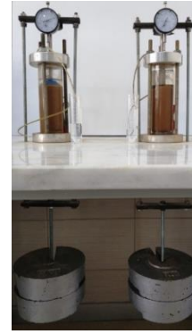
Fig. 3 One-dimensional consolidation stage of samples
