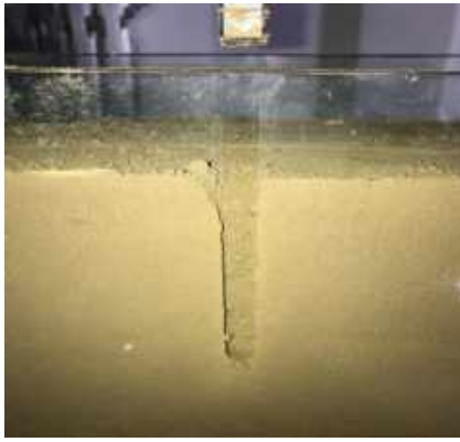
Fig. 15 Soil remains upright after the pile is pulled out
