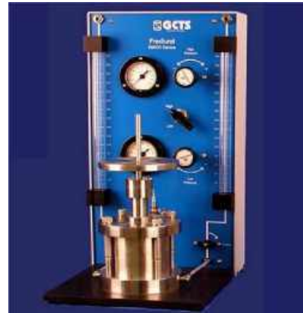
Fig. 1 GCTS SWCC experimental setup
