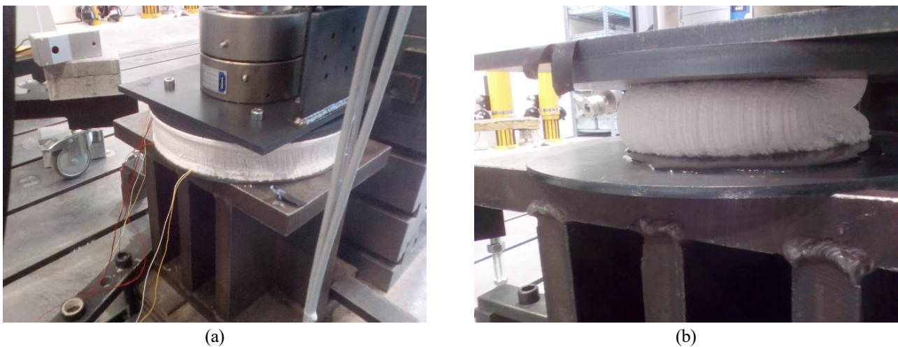
Fig. 6 Deformation and failure mechanisms: (a) Regular sample deformation occurring for lower H/D and (b) Buckling-form deformation occurring at larger H/D
