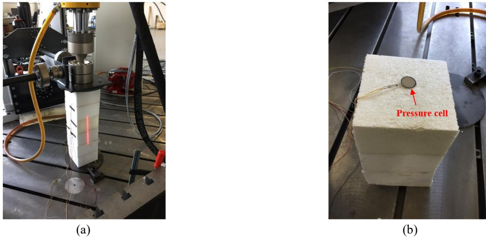
Fig. 3 Measurement devices installed on EPS samples: (a) Different layers of EPS placed in the loading jack and (b) A pressure cell placed on top of the EPS sample
