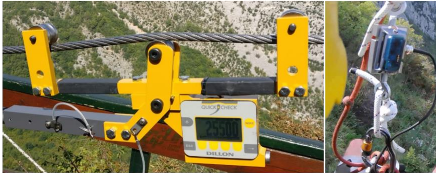
Fig. 4 Tension force measurement due to static loading (left), force and acceleration measurement on the pendulum attachment point (right)
