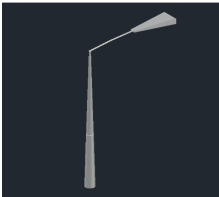
Fig. 2 Schematic representation of lighting pole with variable cross-section cantilever beam
