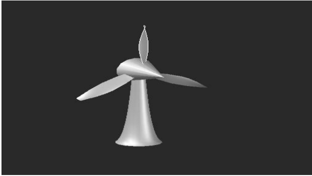
Fig. 1 Schematic representation of wind turbine blades with variable cross-section cantilever beams
