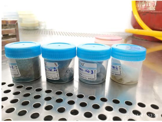
Fig. 5 Sample of fabric with different Cu/ZnO nano-composite loading on fabric
