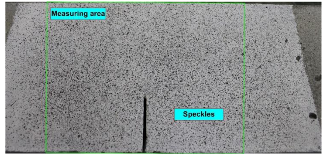
Fig. 2 A view of measuring area of specimen with visible black speckles
