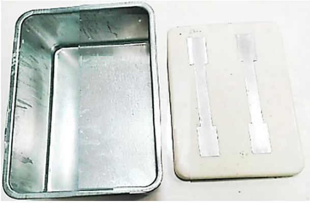
Fig. 2 Construction of mold using dog-bone specimens
