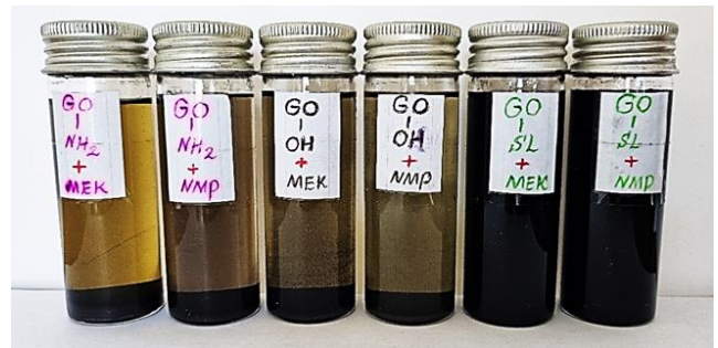
Fig. 12 Image of GO and SGO with different functional groups and SGO in various solvents (After 60 days)
