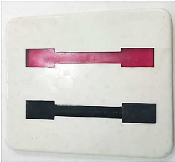
Fig. 4 Molding of pure UPR and NGORP
