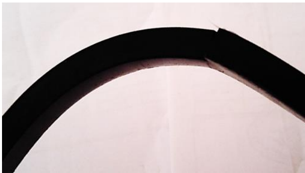
Fig. 8 The flexibility of NGORP-0.15% SGO
