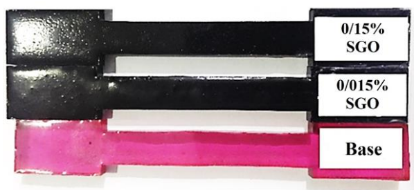
Fig. 9 Shrinkage of the base sample relative to nano-composites
