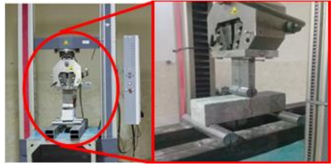
Fig. 2 Sample under fracture energy test
