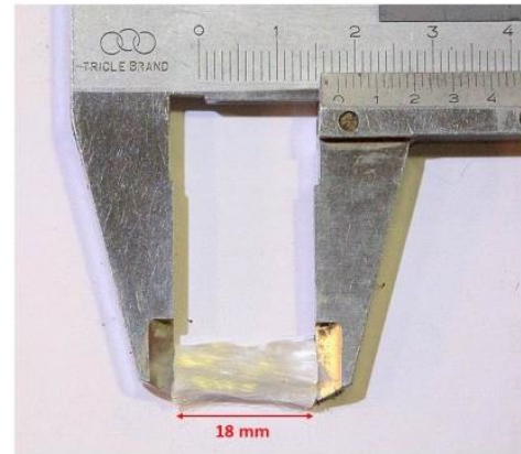
Fig. 8 PP fibers with 18 mm length
