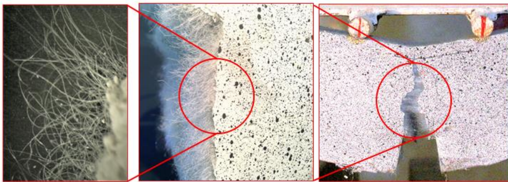
Fig. 19 Pullout of fibers from the matrix through the four-point bending test
