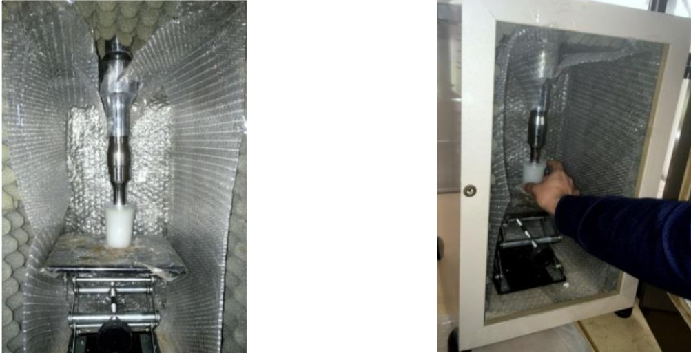
Fig. 9 Sonication of water and NS by an ultrasonic homogenizer
