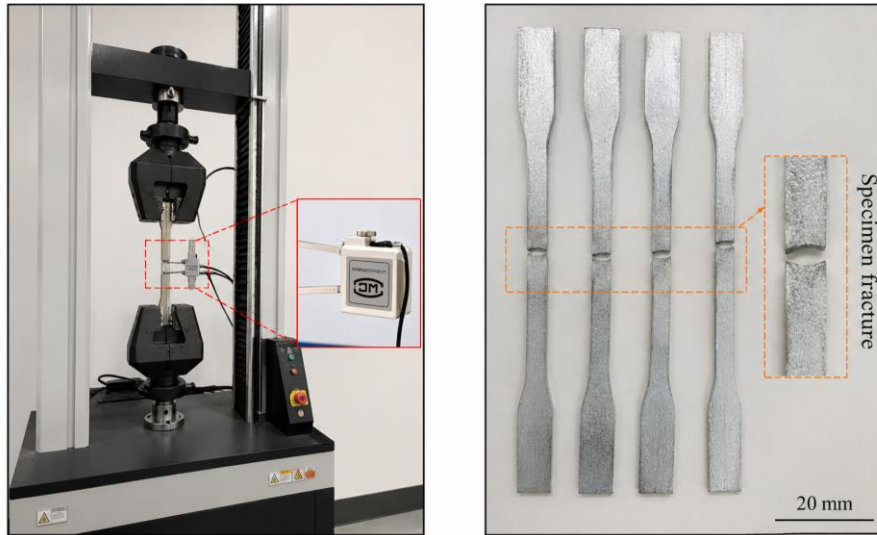
(a) Tensile test machine and extensometer
