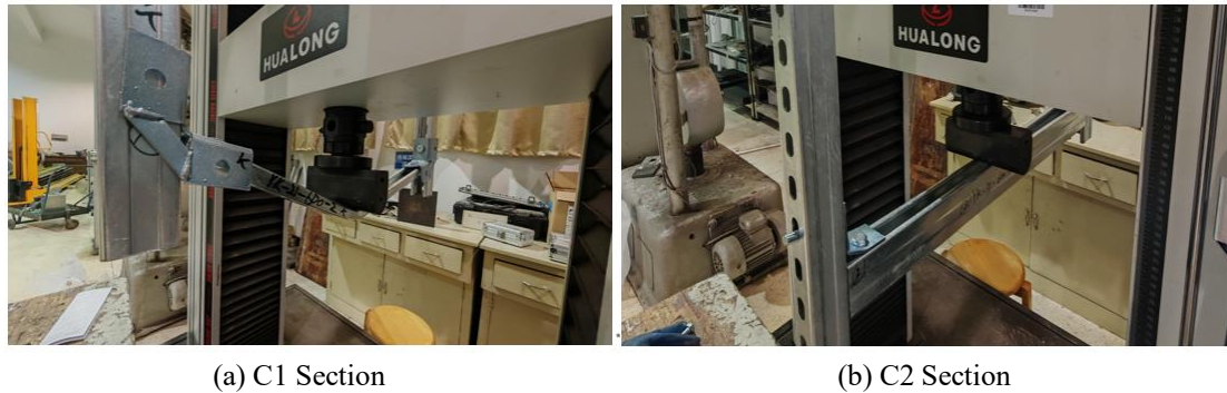
Figure 7. Deformed configuration of the channel steel beam under concentrated loading
