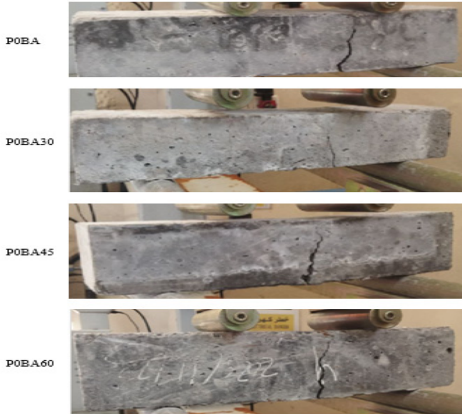
Fig. 9 The crack pattern in the prism beam with 0% recycled plastic
