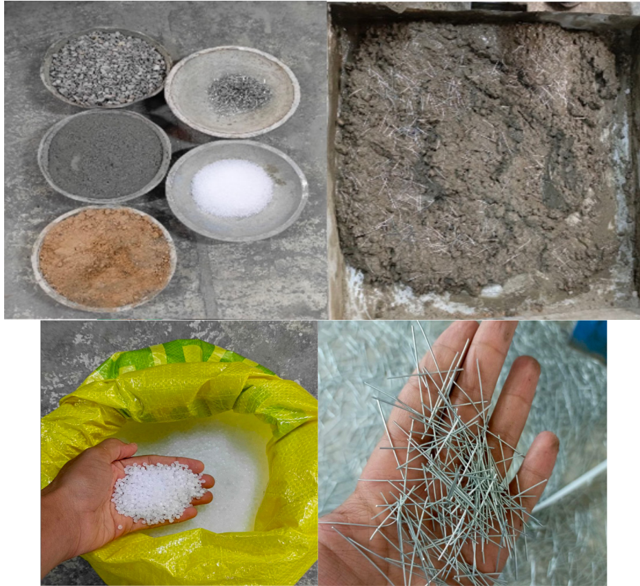
Fig. 1 Prepare material and cast hybrid concrete mixes
