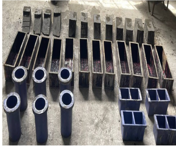
Fig. 2 Prepare and cast recycle concrete samples
