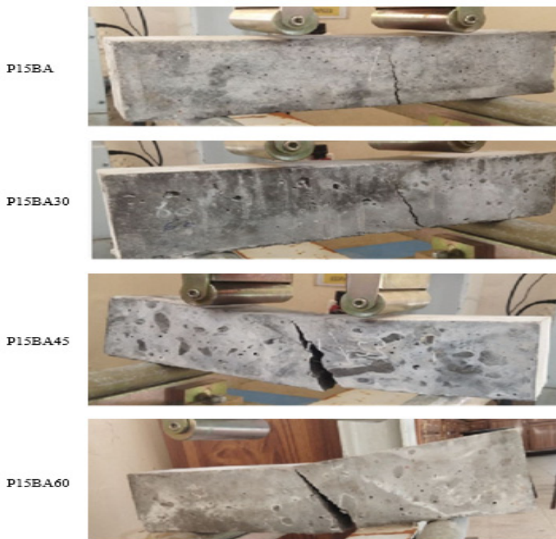
Fig. 12 The crack pattern in the prism beam with 15% recycled plastic
