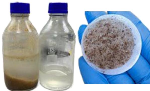
Figure 5. Picture of raw kitchen wastewater (left), treated kitchen wastewater (middle), and fouled membrane (right) [42]
