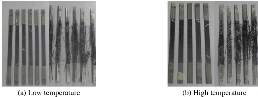
Figure 2. Specimens with 0^\circ fiber orientation due to low and high temperature before (left) and after (right) test
