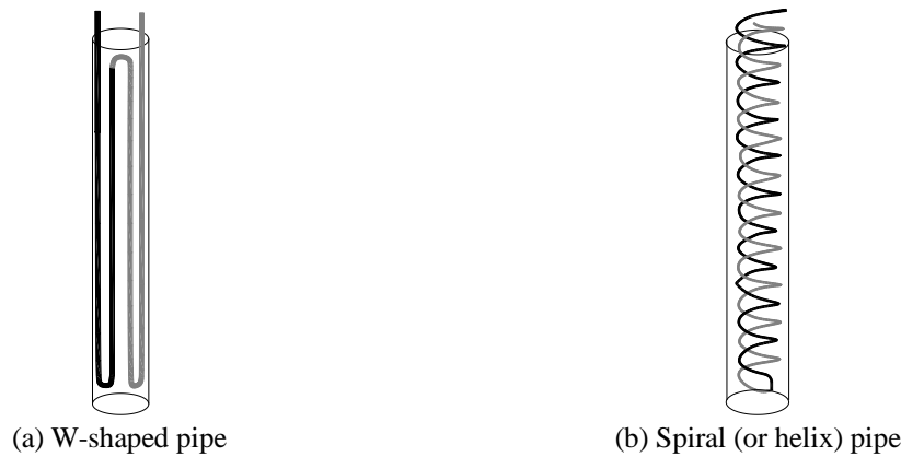
Fig. 2 Two examples of pipe configurations (grey color: inlet, black color: outlet) in energy piles
