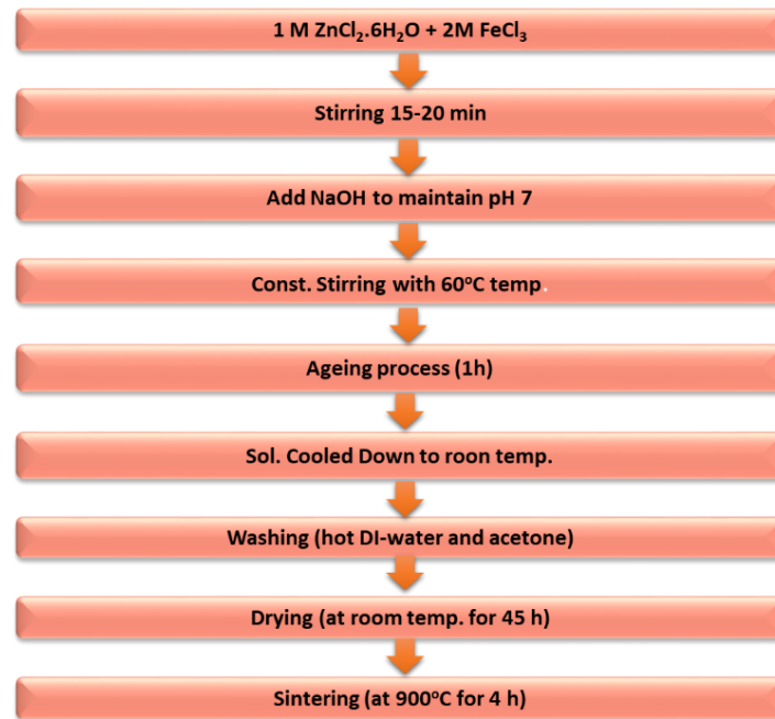
Fig. 5 Flow chart of the synthesis of \text{ZnFe}_2\text{O}_4 nanoparticles prepared by co-precipitation method (a) Andhare et al. (2020)
