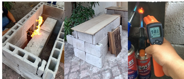
Fig. 4 RC beam inside the fabricated fire furnace
