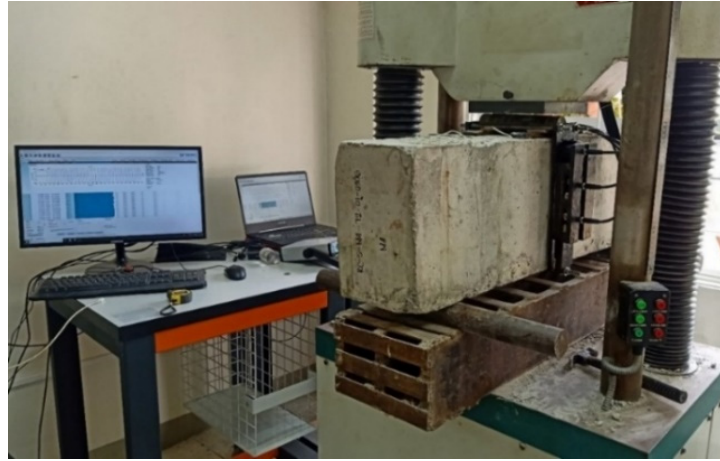
Fig. 5 Destructive flexural test of RC beam while simultaneously measuring the ultrasonic pulses
