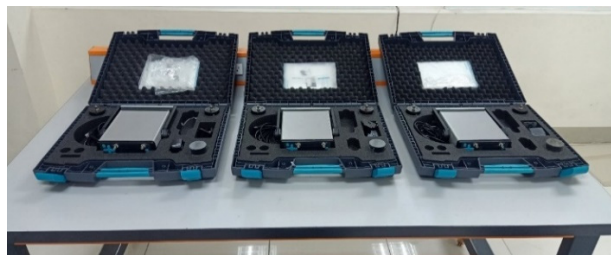
Fig. 3 PUNDIT Lab+ with 54 kHz Ultrasonic Transducers
