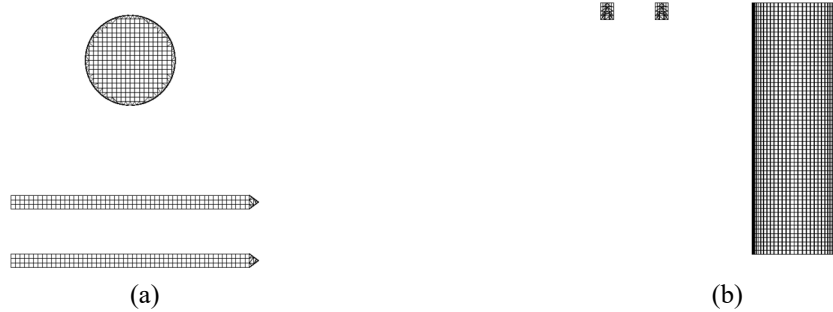
Figure 31. Top view (a) and side view and (b) of panels of catamaran with monopile
