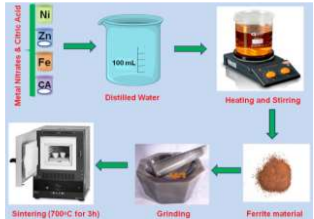
Fig. 1 Synthesis method to prepare powdered samples of highly magnetic Ni-Zn nanoferrites
