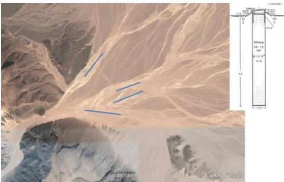
Fig. 3 Infiltration trenches parallel to the stream
