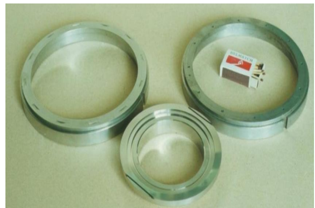
Fig. 4 Rings of friction pairs of mechanical seals
