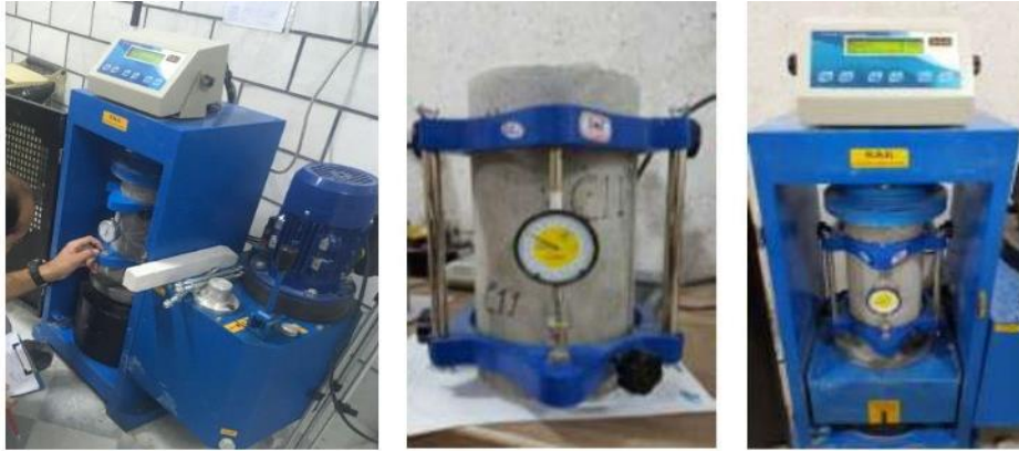
Fig. 7 SME test setup to determine static modulus of elasticity
