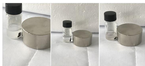
Fig. 9 Attracting magnetite nanoparticles of (a) \text{CoFe}_2\text{O}_4 , (b) \text{CoFe}_2\text{O}_4@\text{SiO}_2 and (c) \text{CoFe}_2\text{O}_4@\text{SiO}_2@[\text{BMIM}]\text{PF}_6 by a magnet (Zhang et al. 2019c)
