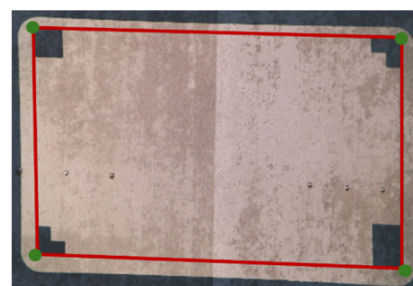
Fig. 5 Examples of detected corners (Green Circle) of the projected pattern
