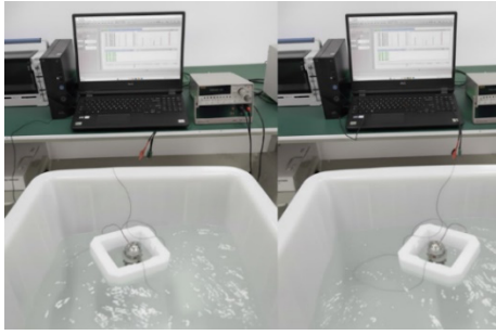
Fig. 3 Experimental setup for testing the smart spherical harvester
