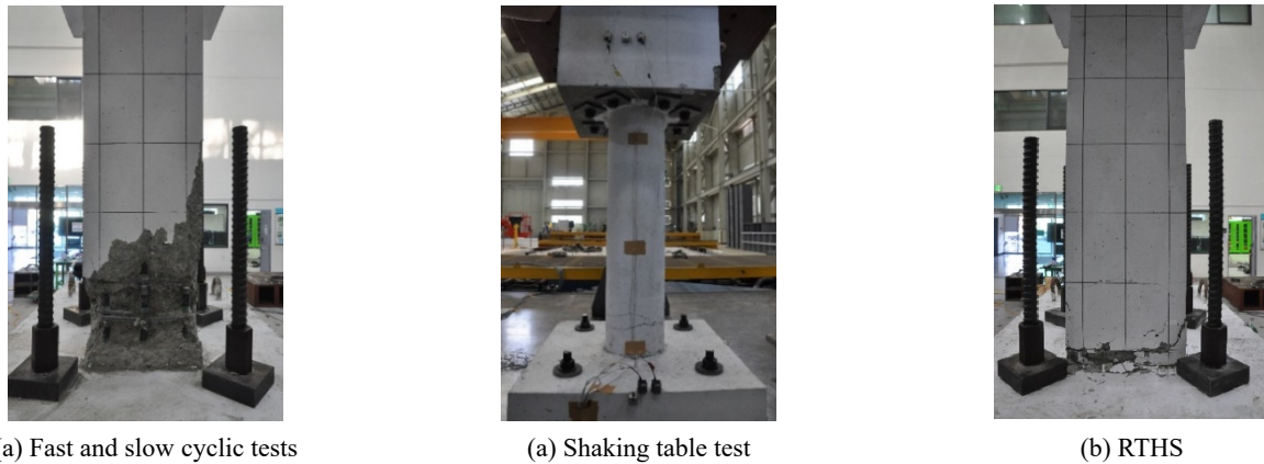
Fig. 1 Bridge pier experiments under different loading protocols
