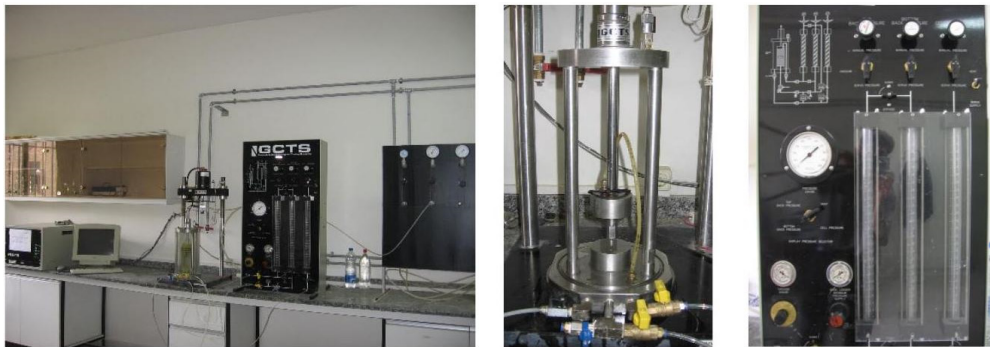
Fig. 1 GCTS triaxial apparatus used in study
