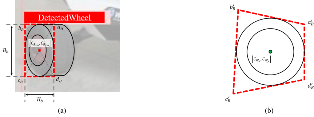
Fig. 5 Detected bounding box correction for wheel center localization (a) illustration of bounding box; (b) corrected bounding box geometry
