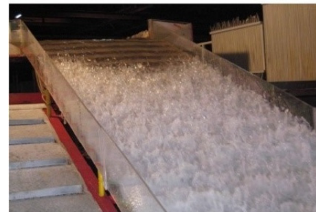
Fig. 14 The results of the flow type in the hydraulic model with a discharge of 92 cubic meters per second (2006)
